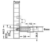
· Area of application: For stabilising the panel against buckling when pulling out the drawer
