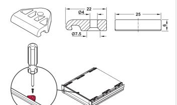
· Area of application: For stabilising the panel against buckling when pulling out the drawer
